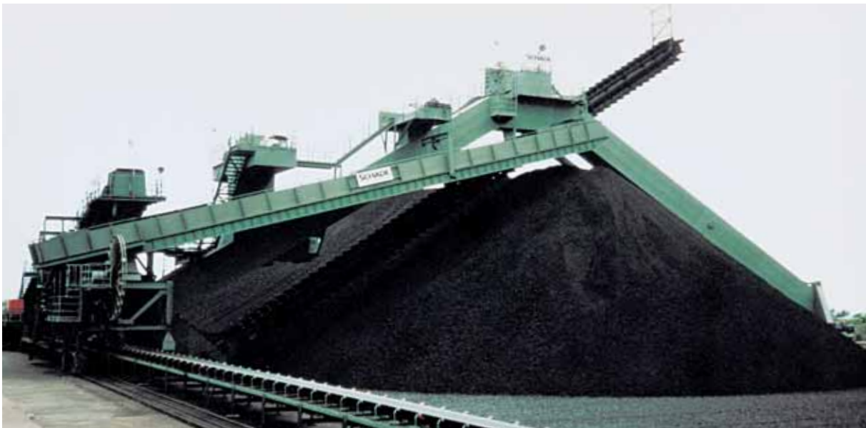
Combined Stacker Reclaimer, 46 m span, stacking 600t/h, reclaiming 300t/h, coal
