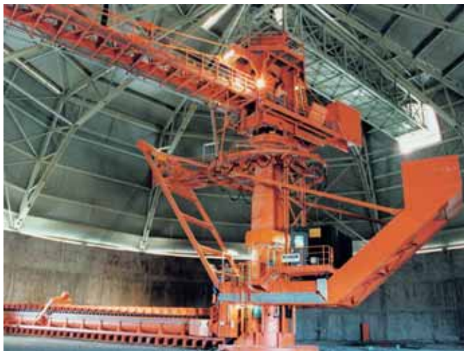
Circular Stacker / Cantilever Scraper Reclaimer, dia 61 m, stacking 1,700 t/h, reclaiming 2,500 t/h, iron ore concentrate
