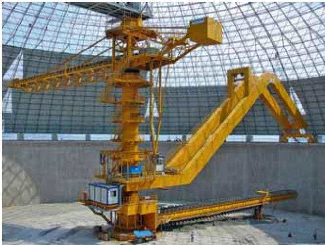
Circular Stacker / Semiportal Scraper Reclaimer, dia 120 m, stacking 3,000 t/h, reclaiming 1,500 t/h, coal
