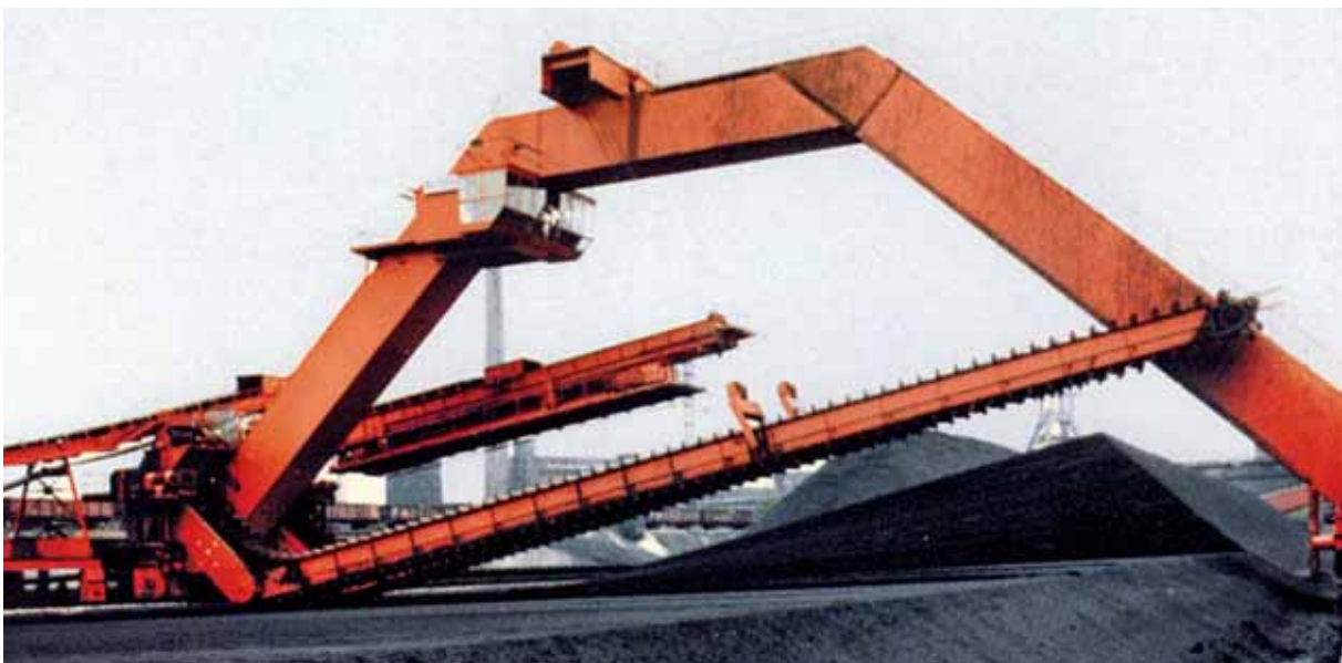
Combined Stacker Reclaimer, 47 m span, stacking 1,500 t/h, reclaiming 900 t/h, coking coal
