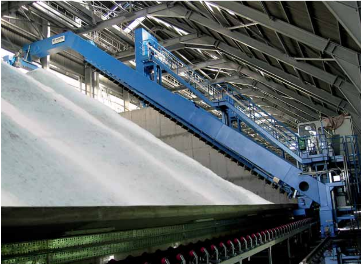
Portal Scraper Reclaimer, 21 m span, 150 t/h, additives
