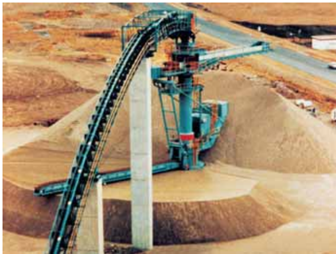
Circular Stacker / Cantilever Scraper Reclaimer, dia 70 m, stacking 1,000 t/h, reclaiming 100 t/h, slag
