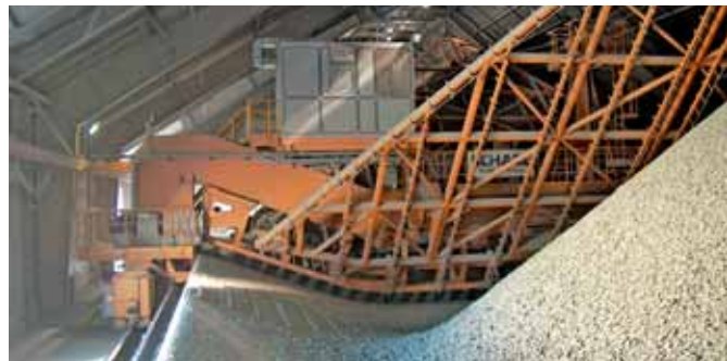
Bridge Scraper Reclaimer, 27,5 m span, 300 t/h, gypsum
