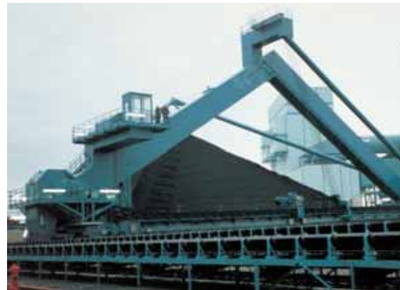
Portal Bridge Reclaimer, 50 m span, 1,225 m³/h for combined storage and blending of various coal qualities
