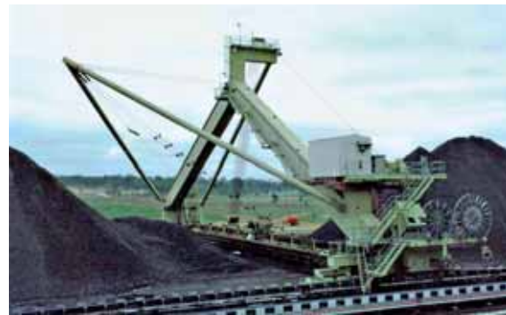
Portal Bridge Reclaimer, 50 m span, 600 t/h, coal
