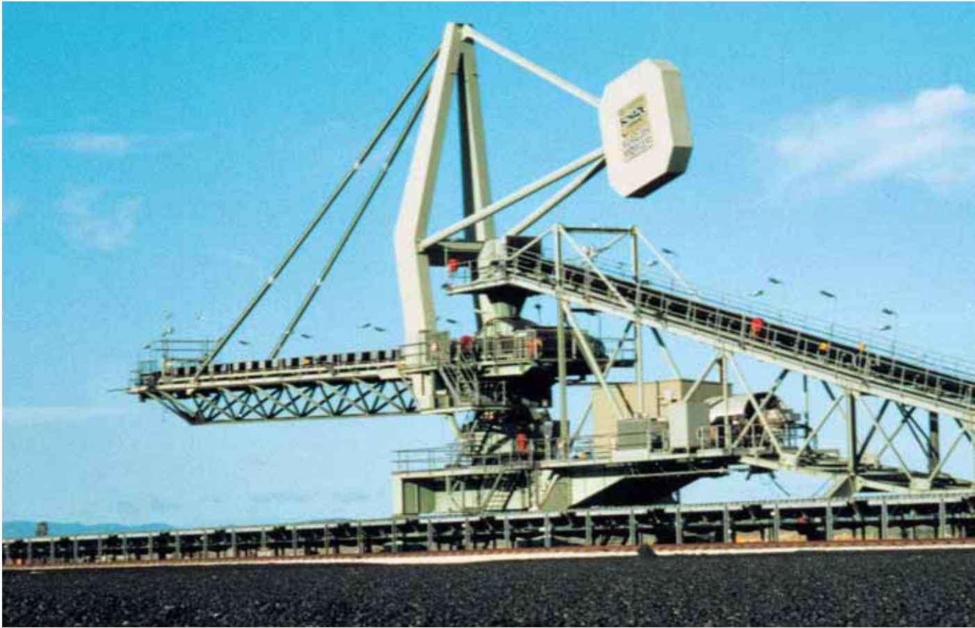
Fig. 1 Slewing/Luffing/Stacker for 2,750 t/h coal
