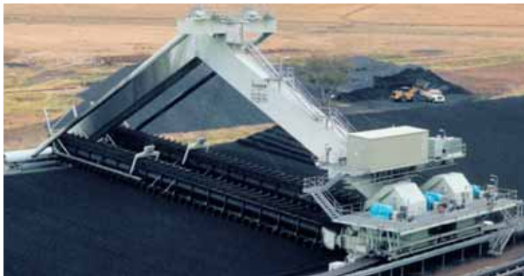
Portal Scraper Reclaimer with twin booms, 52 m span, 3,100 t/h, coal
