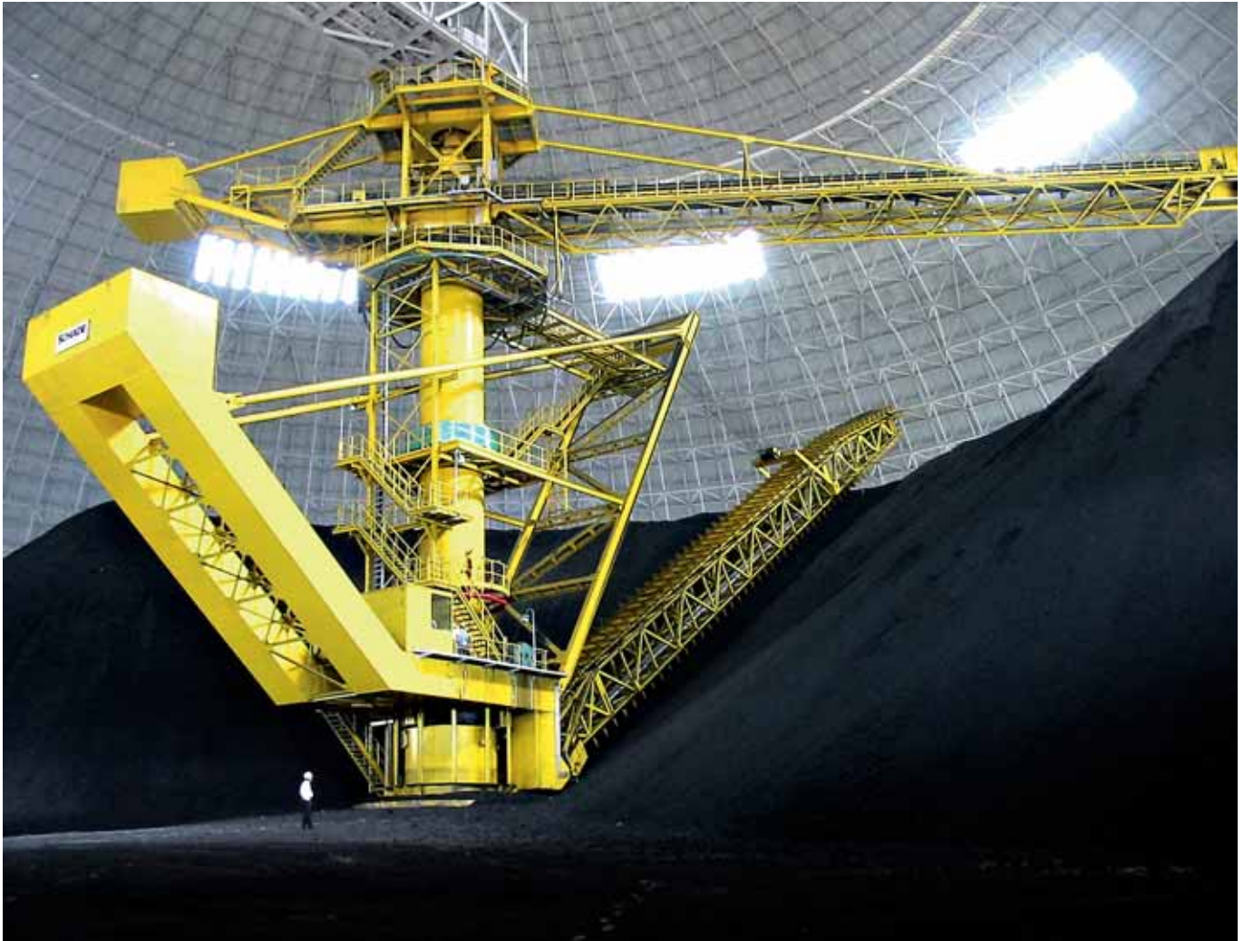
Circular Stacker Cantilever Scraper Reclaimer, dia 120 m, stacking 4,000, reclaiming 2,000 t/h, coal
