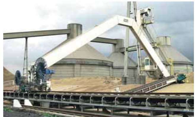
Portal Scraper Reclaimer, 33 m span, 600 t/h, slag
