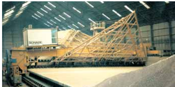
Bridge Scraper Reclaimer, 26,4 m span, 250 t/h, limestone
