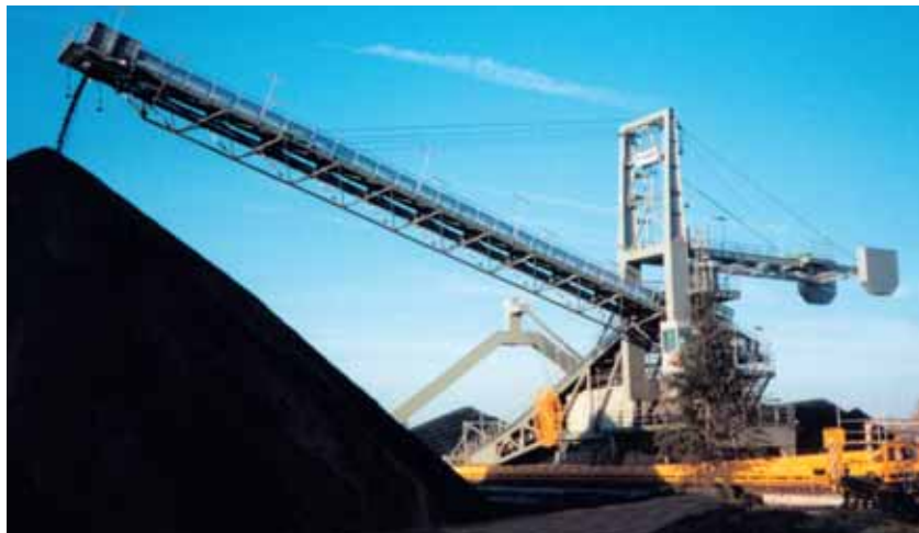
Fig. 2 Slewing/Luffing/Stacker for 1,000 t/h coal
