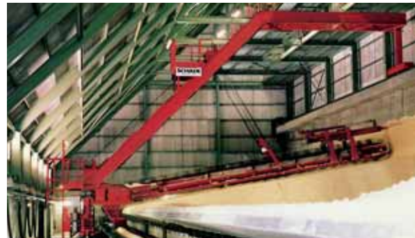
Semi Portal Scraper Reclaimer, 14 m span, 80 t/h, FGD-gypsum
