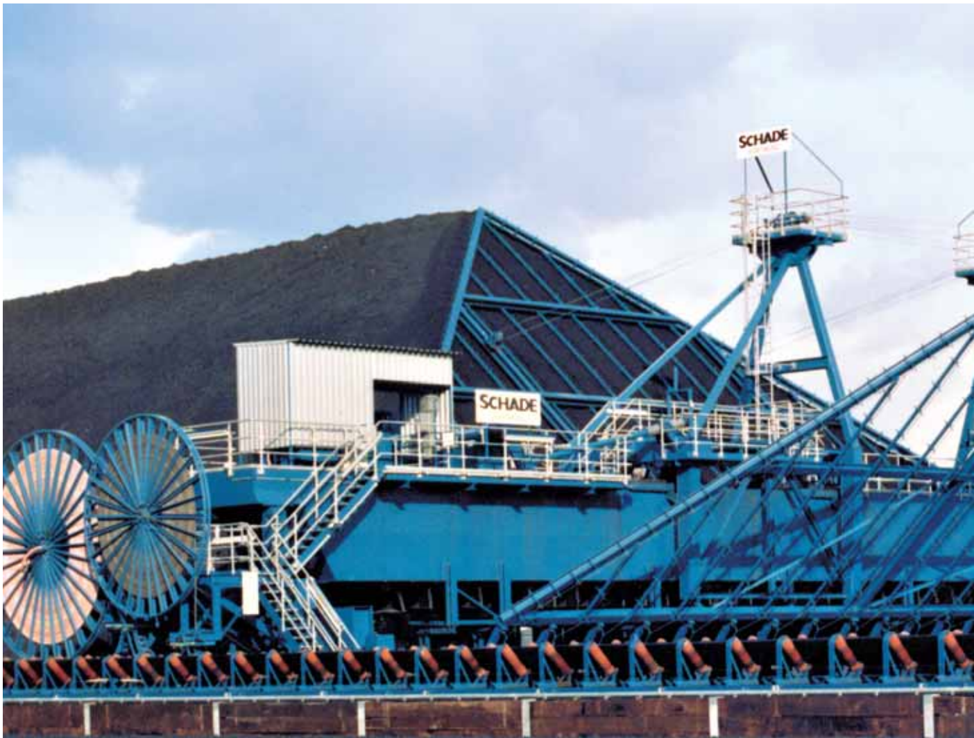
Bridge Scraper Reclaimer, 50 m span, 1,100 t/h, coal
