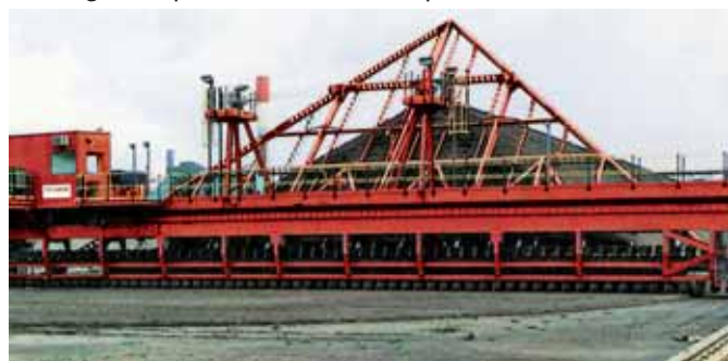
Bridge Scraper Reclaimer, 35 m span, 500 t/h, iron ore
