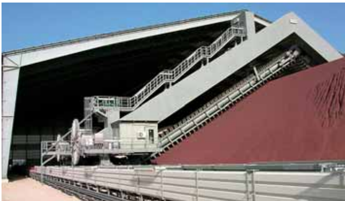
Portal Scraper Reclaimer, 49 m span, 550 t/h, additives
