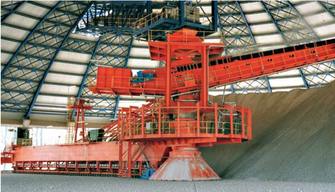
Circular Bridge Stacker / Bridge Scraper Reclaimer, rail dia 78 m, stacking 1,000 t/h, reclaiming 300 t/h, limestone
