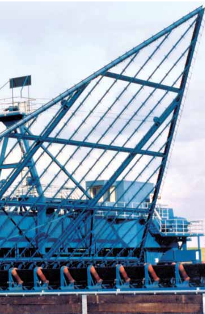
Bridge Scraper Reclaimer, 26,4 m span, 250 t/h, limestone
